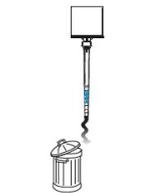
9. Insert the mixing nozzle to the bottom of the hole. Extrude the resin and slowly withdraw the nozzle from the hole. Ensure no air voids are created as the nozzle is withdrawn. Inject resin until the hole is approximately 3/4 full and remove the nozzle from the hole.
